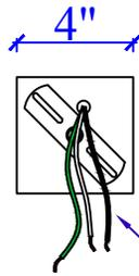
STANDARD 4" ROUND OR SQUARE PANCAKE BOX WITH HANGAR BAR. USE PROPER ANCHOR BOLTS/LAG BOLTS TO SECURE.
