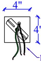
STANDARD 4" ROUND OR SQUARE PANCAKE BOX WITH HANGAR BAR. USE PROPER ANCHOR BOLTS/LAG BOLTS TO SECURE.
