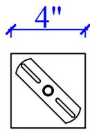
STANDARD 4" ROUND OR SQUARE PANCAKE BOX WITH HANGAR BAR. USE PROPER ANCHOR BOLTS/LAG BOLTS TO SECURE.
