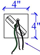
STANDARD 4" ROUND OR SQUARE PANCAKE BOX WITH HANGAR BAR. USE PROPER ANCHOR BOLTS/LAG BOLTS TO SECURE.
