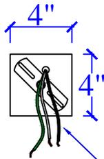
STANDARD 4" ROUND OR SQUARE PANCAKE BOX WITH HANGAR BAR. USE PROPER ANCHOR BOLTS/LAG BOLTS TO SECURE.
