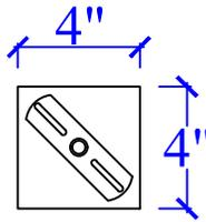
STANDARD 4" ROUND OR SQUARE PANCAKE BOX WITH HANGAR BAR. USE PROPER ANCHOR BOLTS/LAG BOLTS TO SECURE.
