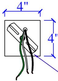
STANDARD 4" ROUND OR SQUARE PANCAKE BOX WITH HANGAR BAR. PANCAKE BOX MUST BE SECURED TO HOLD FIXTURE. USE PROPER ANCHOR BOLTS/LAG BOLTS
