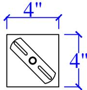
STANDARD 4" ROUND OR SQUARE PANCAKE BOX WITH HANGAR BAR. PANCAKE BOX MUST BE SECURED TO HOLD FIXTURE. USE PROPER ANCHOR BOLTS/LAG BOLTS
