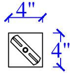
STANDARD 4" ROUND OR SQUARE PANCAKE BOX WITH HANGAR BAR. USE PROPER ANCHOR BOLTS/LAG BOLTS TO SECURE.
