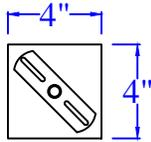
STANDARD 4" ROUND OR SQUARE PANCAKE BOX WITH HANGAR BAR. PANCAKE BOX MUST BE SECURED TO HOLD FIXTURE. USE PROPER ANCHOR BOLTS/LAG BOLTS
